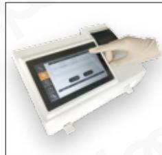
Insert the 1st test and Press "START TEST" as the 1st alarm starts to ring. Repeat the same operation for the rest tests.
