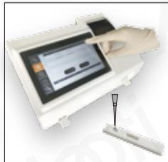
Dispense the 1st sample and Press "START INCUBATION". Repeat the same operation for the rest tests.
